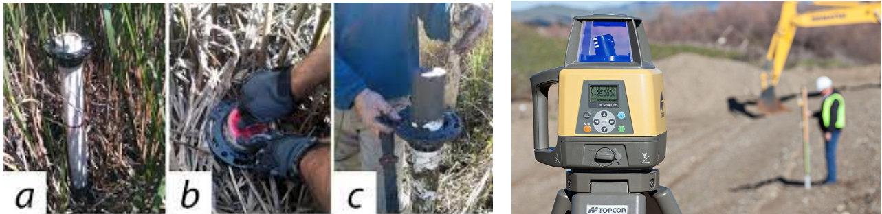
Figure 1. Left: An example of a PVC pipe as the coring tool, which is then used as the storage container for the sample. Right: Tool set that measures elevation using a laser beam and a reflector.
